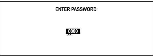
You must enter your secure password to access the next screen. The position of each of the four digits of the password is indicated by the mark below the zero. The system will remain password free for five minutes, allowing changes to be made.
